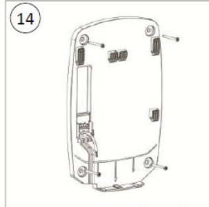
14 Screw the Plug-in base to the wall(x4)
