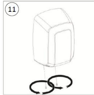
11 Screw the cover fixing screws (x2) Your dryer is now ready to be used on
