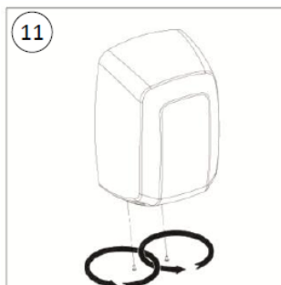
11 Screw the cover fixing screws (x2) Your dryer is now ready to be used on a Plug-in base
