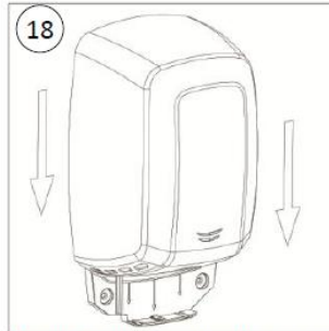
18 Mount the dryer over the Plug-in base with a from top to down movement
