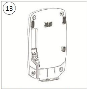
13 Route the wires through the Plug-in base as shown on the picture
